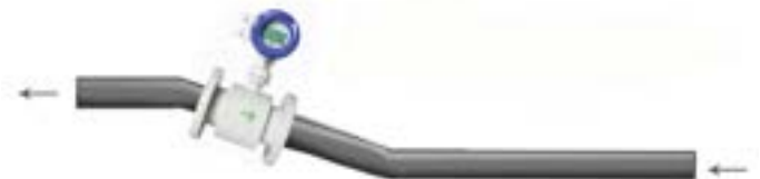
Install at the rising direction
