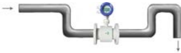
Install at the lowest point when used in open drain pipe
