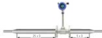
Concentric Expansion Pipeline
