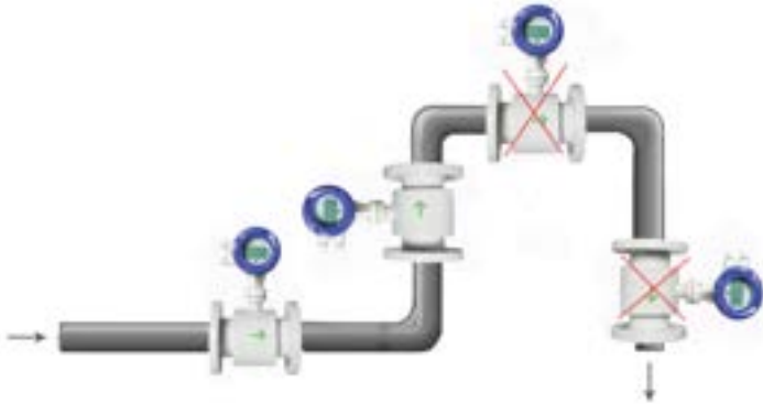
Install at the lowest point and vertical upward direction
