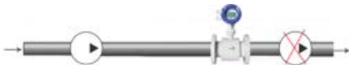
Dont' install it at the entrance of pump, install it at the exit of pump
