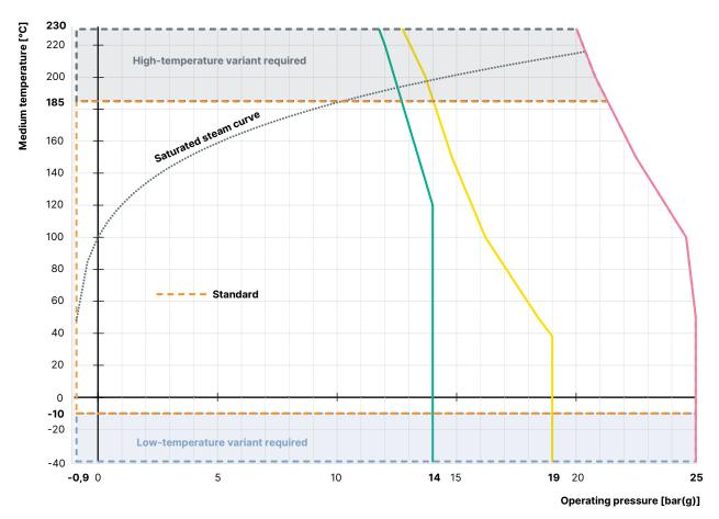
Operating limits for PN25 according to DIN EN 12516-1
