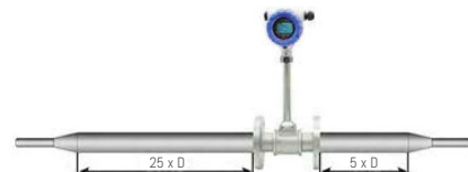
Concentric Expansion Pipeline
