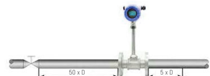
Regulating Valve, Half-open Gate
