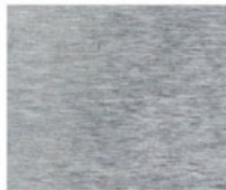
Surface finish: fine-machined, and grinded, Ra 0.4 \mu\text{m}
