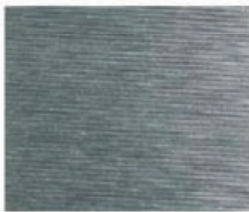
Surface finish: machined, Ra 1.2 \mu\text{m}
