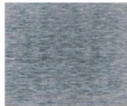
Surface finish: fine-machined, and grinded, Ra 0.2 \mu\text{m}
