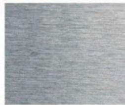
Surface finish: machined, Ra 0.8 \mu\text{m}
